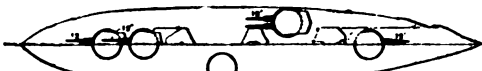
Great Britain. Battleship of the Neptune Class Length 510 ft.; 19,900-20,000 tons; speed 21.5-21.78 knots; armament 10-12 in., 16-4 in., 4-3 pr., 5 small. Completed 1911.
